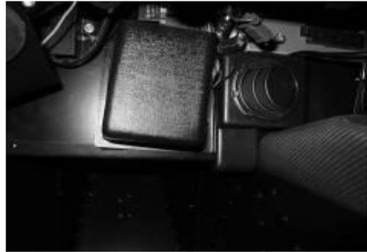
If you have a metal fuse box cover as per the picture, fit edge trim to the top of the cover and any other 'non-radiused' edges.
