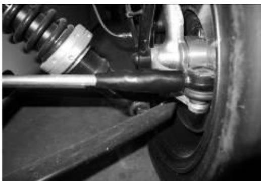
Check all plastic covers are fitted to the front suspension bolt. Also fit to the exhaust mounting bolt heads and (if fitted) rollcage mounting bolt heads.
