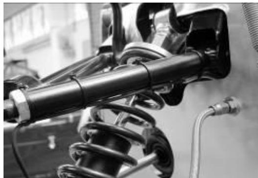
...and that there is some washer pipe where the wire passes into the body work (to protect against chaffing). The pipe can be split with a knife to allow it to be added to the wire.
