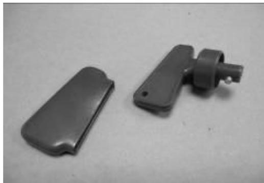
Check that rubber covers are fitted over the track rod ends and lock butts. Note: The 'blind' end of the cover will need to be cut off to fit over the track rod arm.
