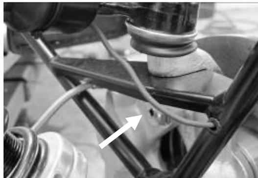
Ensure the side repeater wiring is neatly and securely clipped to the wishbone...
