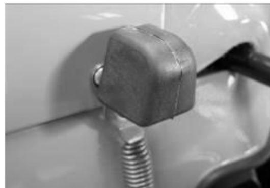
Bend the exhaust spring mounting hooks down and put some washer pipe over the end.
