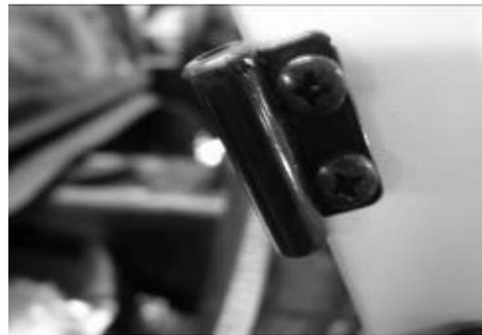
Ensure large grommets are fitted to the knee trim panels under the dash on either side.
