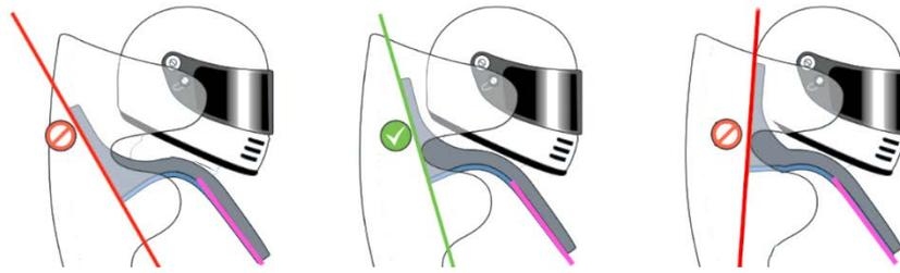
Figure 2 Examples of incorrect and correct HANS® angles
