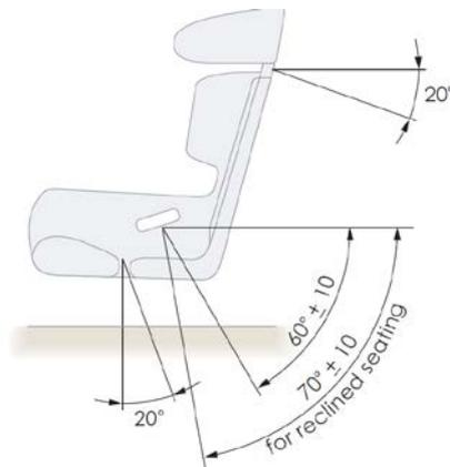
**Figure 13 Side view to show recommended belt angles**
