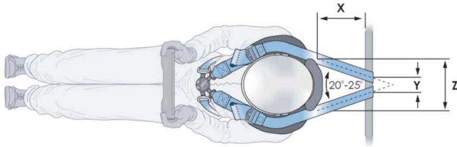
**Figure 12 Position of shoulder belt anchorage points to achieve desired belt angle (plan view)**
