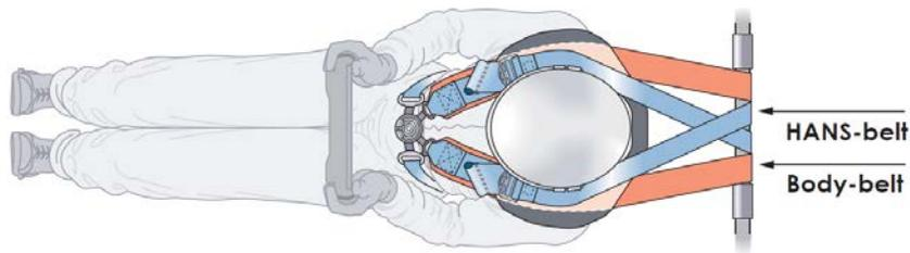
**Figure 16 Installation of HANS double belts in cars where ( $X > 200\text{mm}$ )**
