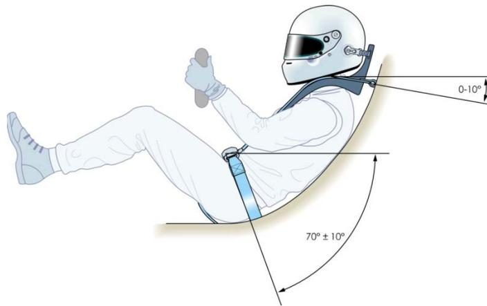
Figure 14 recommended belt angle for open cockpit cars
