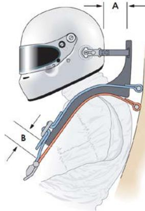
**Figure 11 Minimum distance between HANS-yokes and double-shoulder belt merge point**
