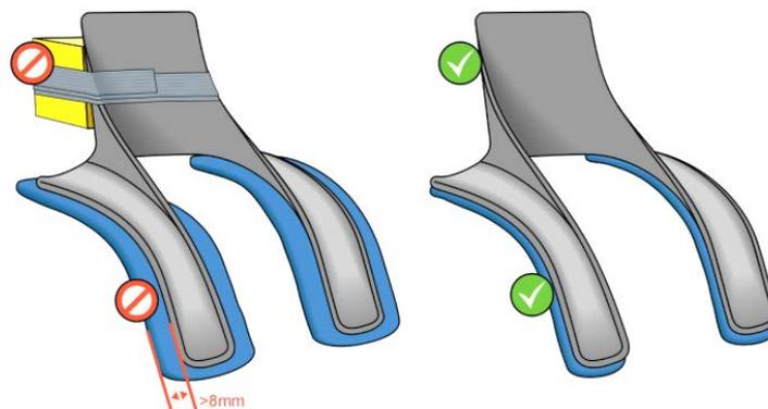
Figure 6 Examples of incorrect and correct HANS® padding
